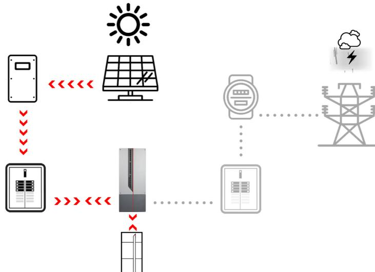
**Figure 4 – AC-Coupled Current Flows with Sufficient Load or Charging Demand**
