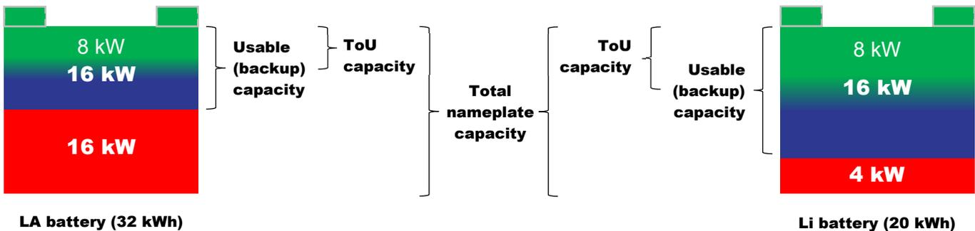
**Figure 9 – Capacity Levels for Batteries**
